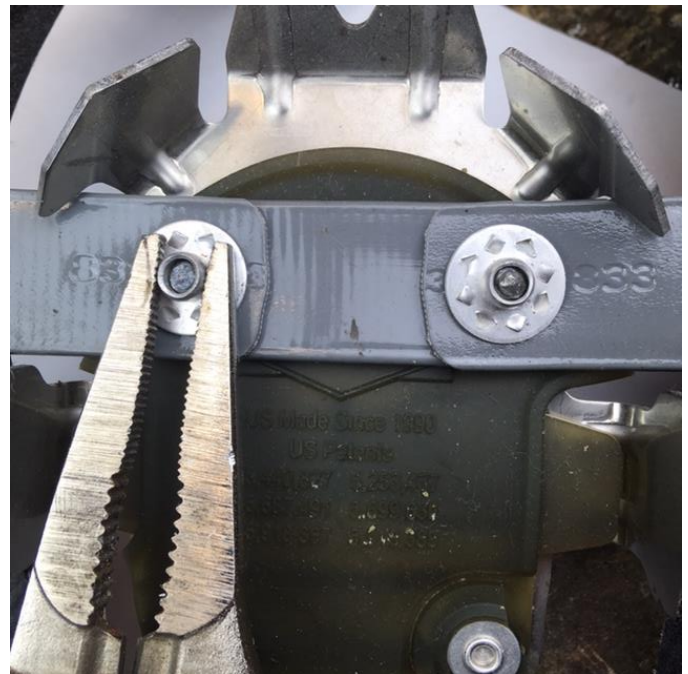
View: Bottom of snowshoe. Using pliers to hold bottom of rivet to prevent spinning while drilling out rivet
