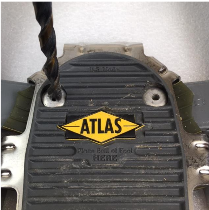
View: Top of snowshoe- Aluminum Rivet
