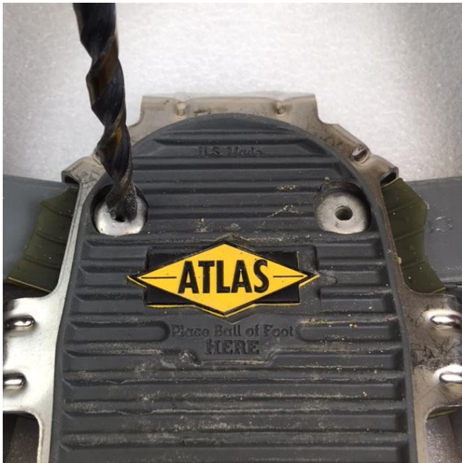
Top of snowshoe- Aluminum Rivet
