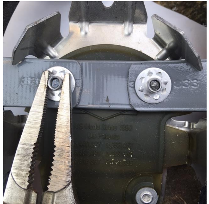
Using pliers to hold bottom of rivet to prevent spinning while drilling out rivet
